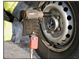
WHC work with Severn Trent Water to ensure they supply them with the highest quality tools with the lowest vibration frequency possible. Their test engineers are all IOSH trained for vibration testing by an IOSH recognised company. Alongside this WHC modify STW's equipment to reduce the vibration levels by upgrading things such as bushes and dampeners to ensure they get the best performance and lowest vibration levels possible.
