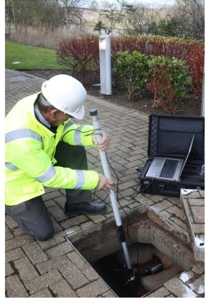
The technology is able to indicate asset condition, with an immediate Red, Amber, Green to the operator. survey results are analysed by NRW's Acoustic Innovations Team to confirm serviceability and recommend the appropriate intervention, where necessary.
